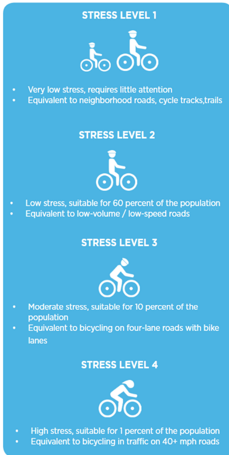
Figure 10: Levels of Traffic Stress. From the Montgomery County, MD Bicycle Master Plan, 2018
