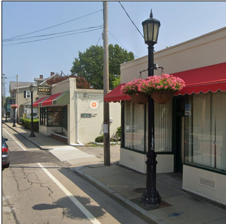
Image 3- Light Posts and Utility Poles Reducing Travel Path Width
